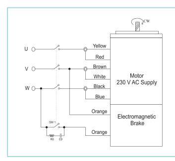
When SW1 is switched ON, electromagnetic Brake is released & motor starts rotating. When Sw1 is switched OFF then electromagnetic brake will be applied stopping motor immediately, holding the load.
