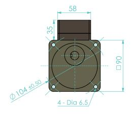
Motor Round Shaft with Terminal Box
